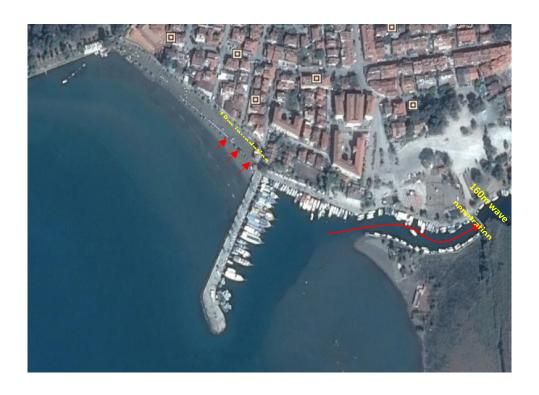
Figure 6.2: Schematic view of wave inundation at Akyaka Beach
