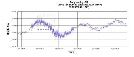
Figure B.O.3: Bodrum Tide Gauge and IDSL Buoy Readings
