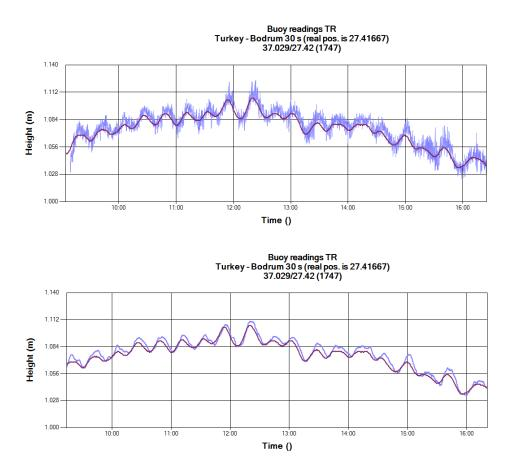
Figure B.O.4: Comparison of Bodrum Tide Gauge and IDSL Buoy Readings
