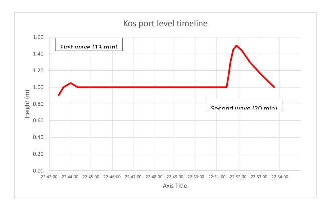
Figure 7.19: The analysis of the images and once corrected for the time delay, the plot represents the absolute height of the water, considering the location of the plant box (1 m from sea level) and the height of the plant box (46 cm). Then, the maximum 1.5 m, at the location of the plant box, occurs at 22:51 UTC but two distinct waves are present, 13 and 20 min after the earthquake.
