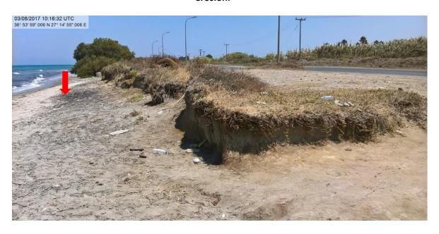
Figure 7.3: Image taken at 36.90433/27.25805. One witness, point (3), reported that the beach was inundated by 16 m and corresponding to 0.5 m water height.
