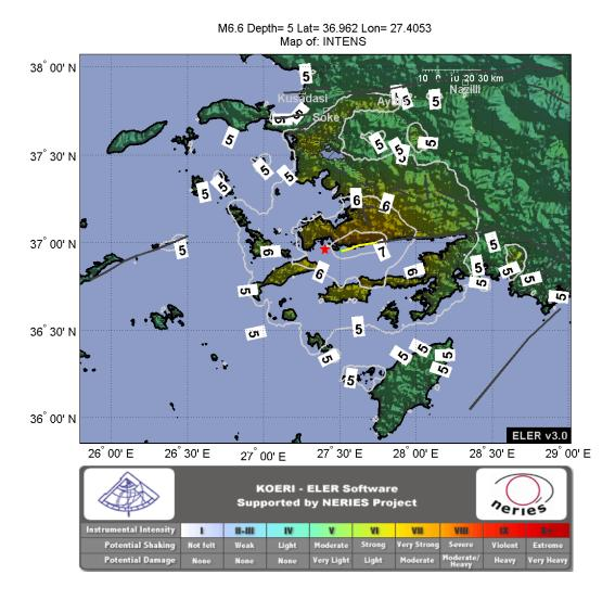
Figure 2.2: Earthquake Intensity Map produced by ELER (KOERI) (M6.6) (Source: ELER-v3.1:
