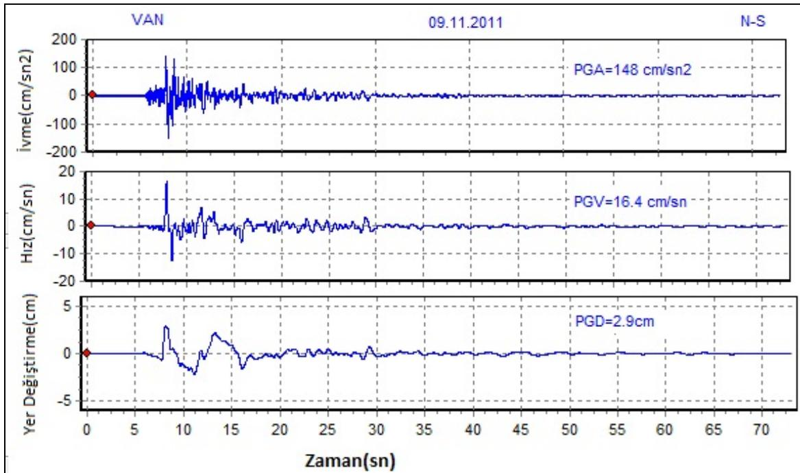
Figure 11.7: NS direction acceleration, velocity and displacement components for 09 November 2011, Ml=5.6 Van-Edremit Earthquake (Van-Merkez station)
