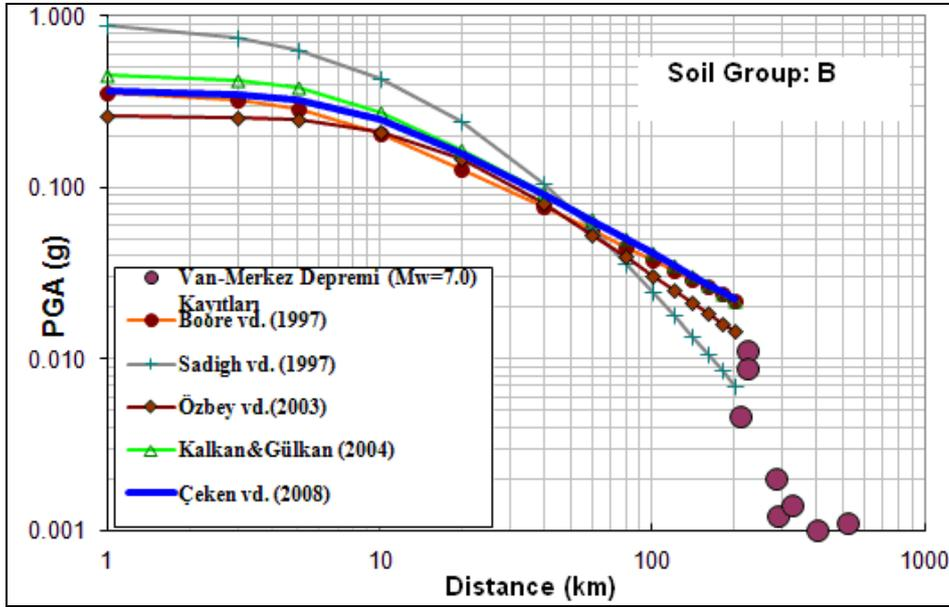
Figure 16.1: Compare with peak ground horizontal acceleration value and some attenuation relationship for 23 October 2007  $M_w=7.0$  Van-Merkez earthquake(soil group:B)
