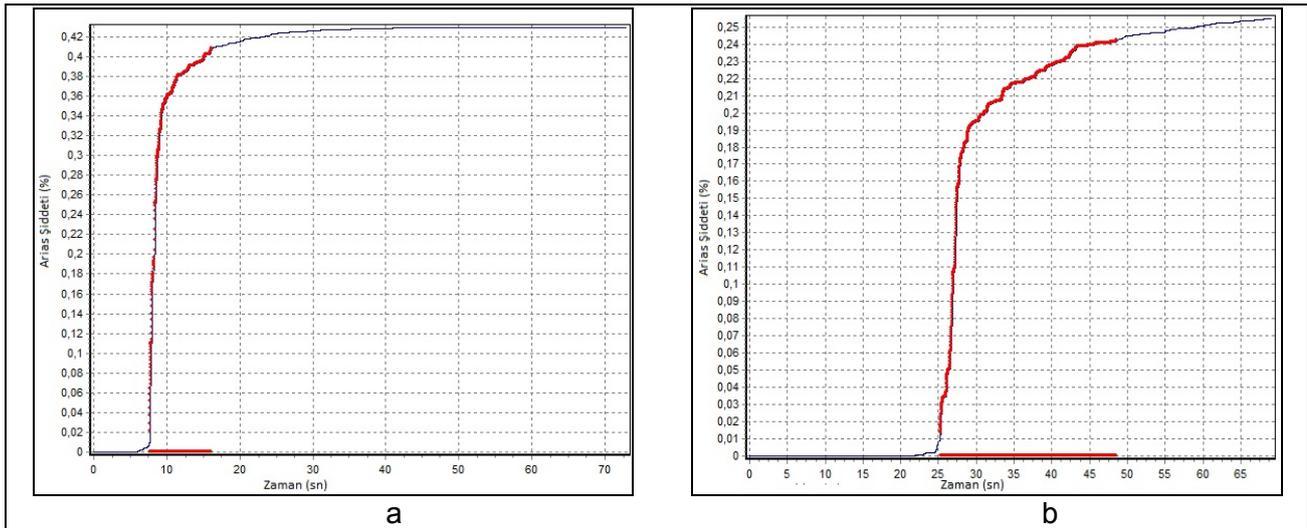
Figure 12.2: 09 November 2011  $M_I=5.6$  Van-Edremit Earthquake effective durations a) Van station record E-W direction, b) Van-Edremit station record E-W direction.
