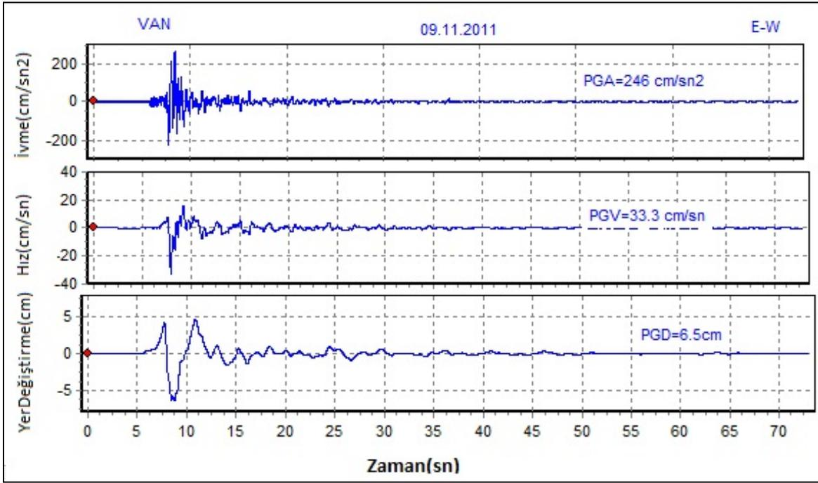
Figure 11.8: EW direction acceleration, velocity and displacement components for 09 November 2011, Ml=5.6 Van-Edremit Earthquake (Van-Merkez station)
