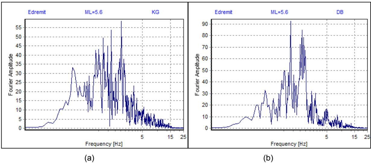
Figure 13.4: Fourier spectrums of 09 November 2011, ML=5.6 Van-Edremit earthquake
