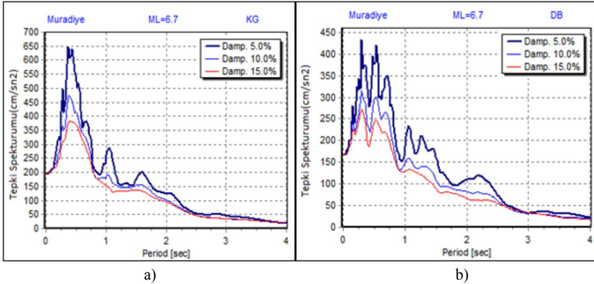
Figure 14.1: Response spectrums of 23 October 2011,  $M_L=6.7$  Van-Merkez earthquake
