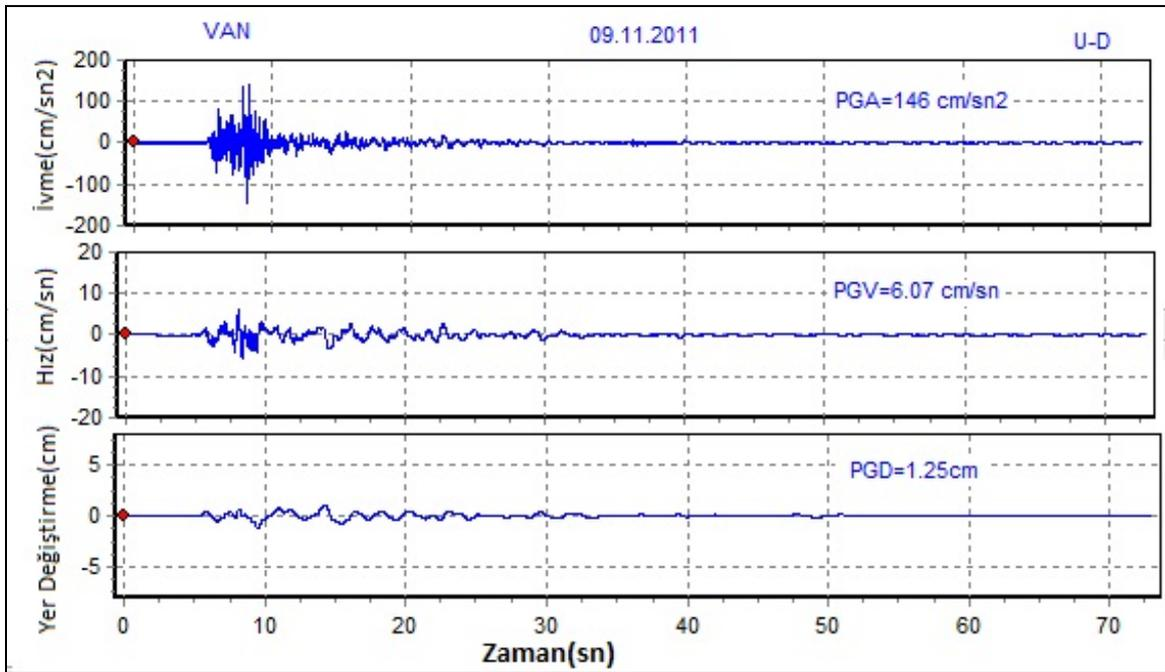
Figure 11.9: Vertical direction acceleration, velocity and displacement components for 09 November 2011, Ml=5.6 Van-Edremit Earthquake (Van-Merkez station)
