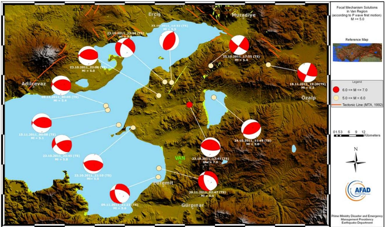
Figure 3.2: Focal mechanism solutions of  $M \geq 5$  earthquakes (according to P wave first motion)
