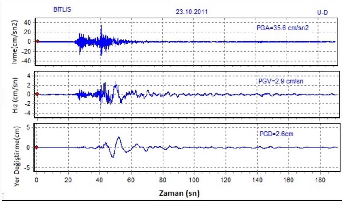
Figure 11.6: Vertical direction acceleration, velocity and displacement components for 23 October 2011, Ml=6.7 Van-Merkez Earthquake (Bitlis station)
