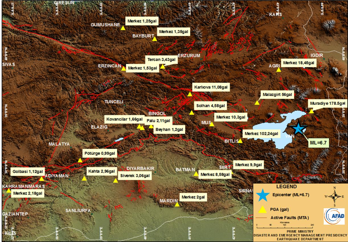
Figure 10.1: Distribution of the recorded stations and peak ground accelerations for 23 October 2011, ML=6.7, Mw=7.0 Van Earthquake.
