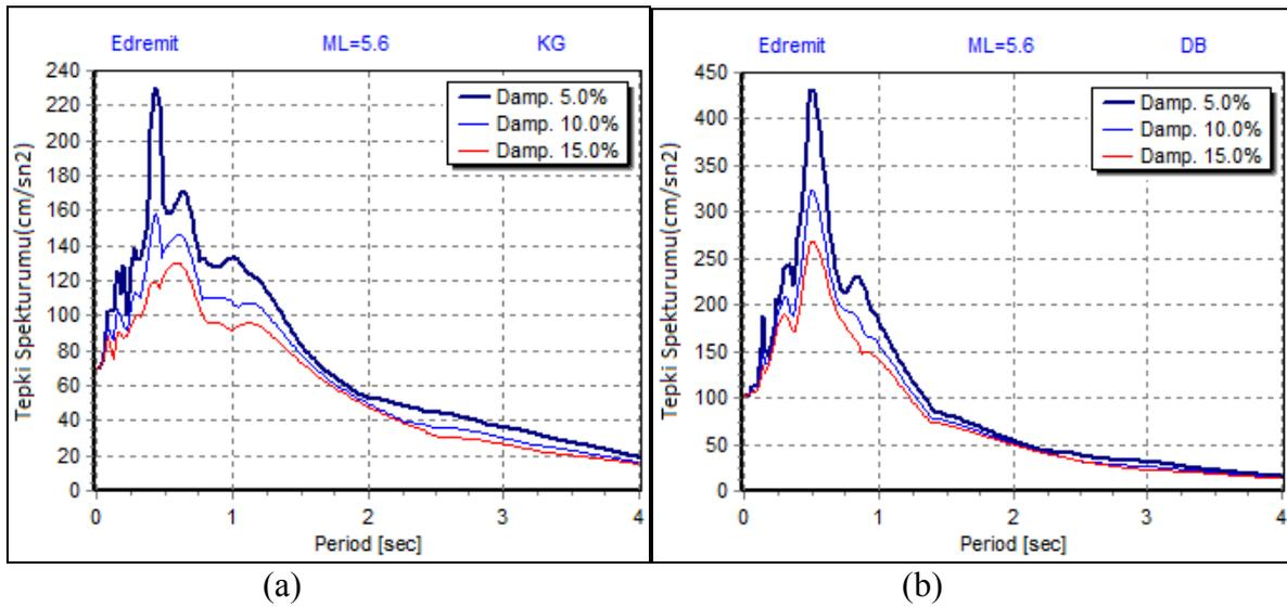
Figure 14.4: Response spectrums of 09 November 2011, ML=5.6 Van-Edremit earthquake
