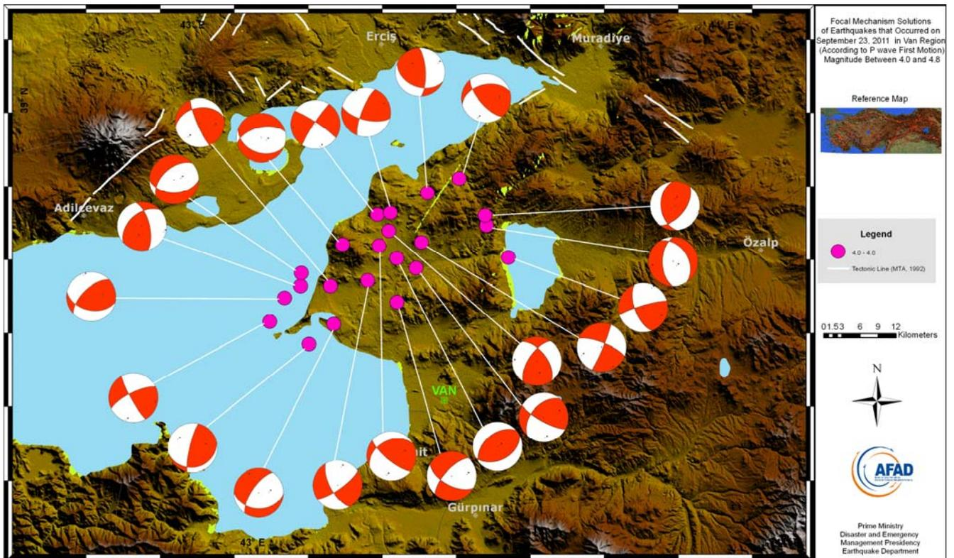
Figure 3.3: Focal mechanism solutions of some earthquakes magnitude between 4 and 4.8 (according to P wave first motion)
