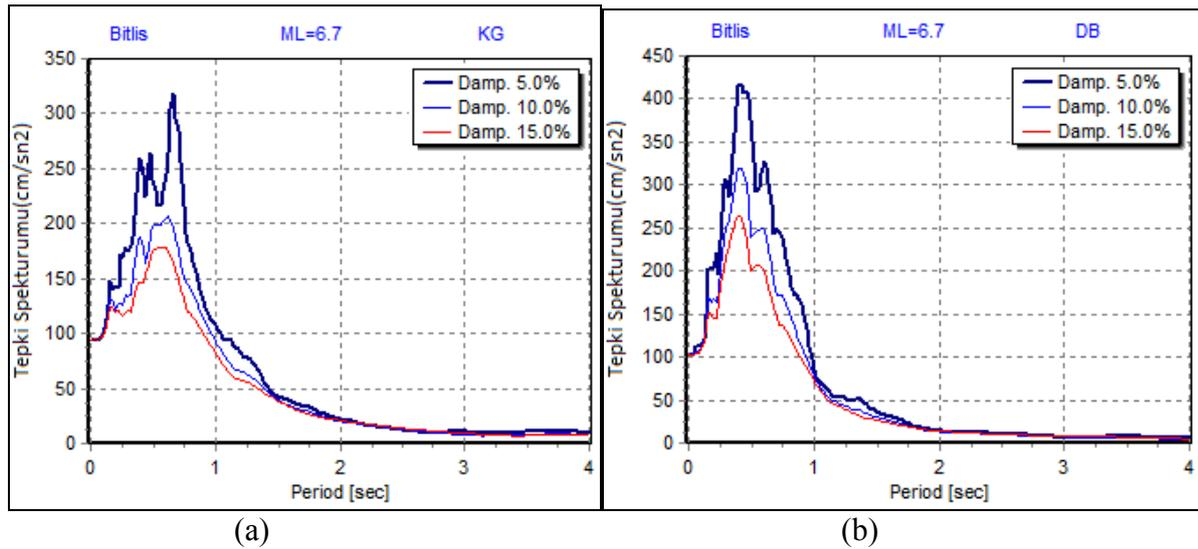
Figure 14.2: Response spectrums of 23 October 2011,  $M_L=6.7$  Van-Merkez earthquake
