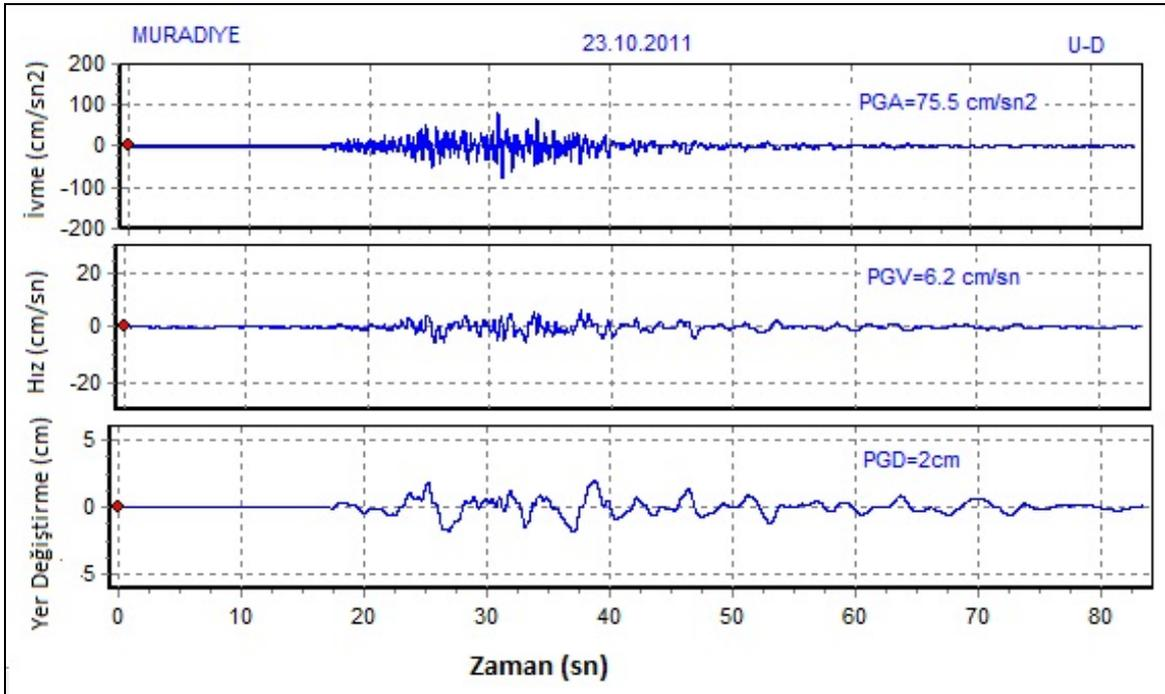
Figure 11.3: Vertical direction acceleration, velocity and displacement components for 23 October 2011, Ml=6.7 Van-Merkez Earthquake (Muradiye station)
