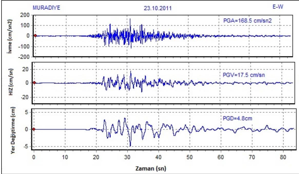
Figure 11.2: EW direction acceleration, velocity and displacement components for 23 October 2011, Ml=6.7 Van-Merkez Earthquake (Muradiye station)
