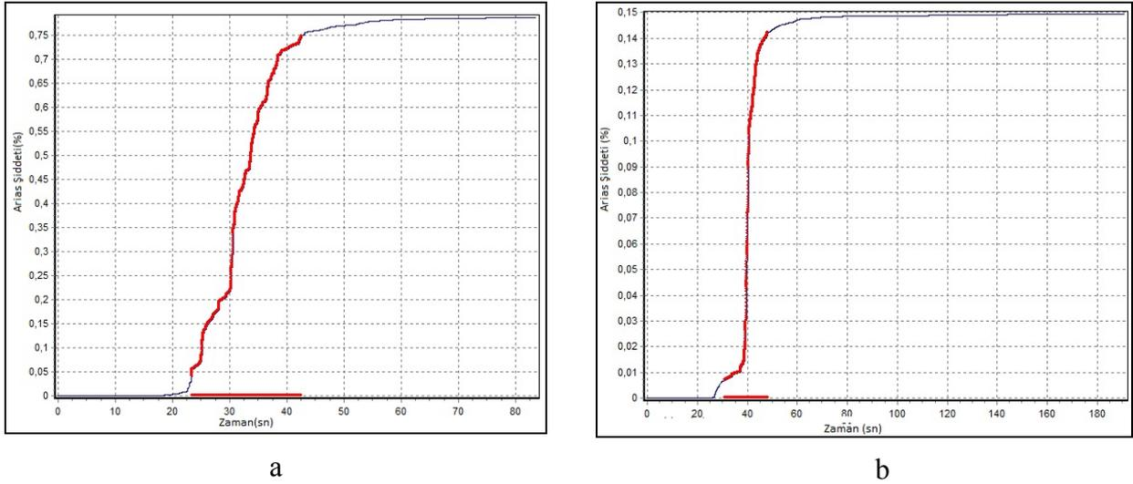
Figure 12.1: 23 October 2011  $M_I=6.7$  Van-Merkez Earthquake effective durations a) Muradiye station record N-S direction, b) Bitlis station record E-W direction.
