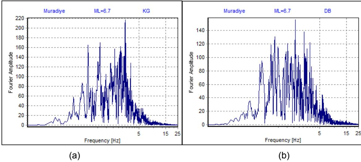
Figure 13.1: Fourier spectrums of 23 October 2011,  $M_L=6.7$  Van-Merkez earthquake
