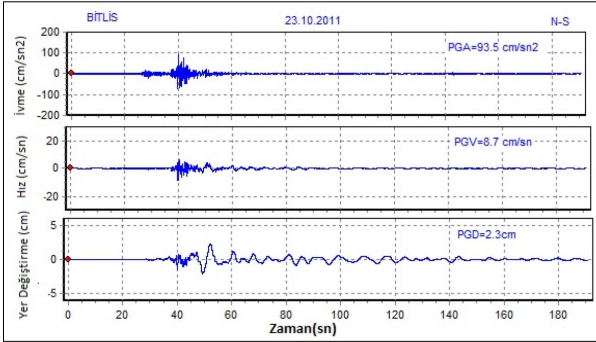
Figure 11.4: NS direction acceleration, velocity and displacement components for 23 October 2011, MI=6.7 Van-Merkez Earthquake (Bitlis station)
