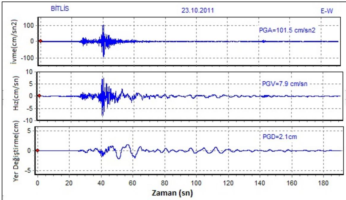
Figure 11.5: EW direction acceleration, velocity and displacement components for 23 October 2011, MI=6.7 Van-Merkez Earthquake (Bitlis station)
