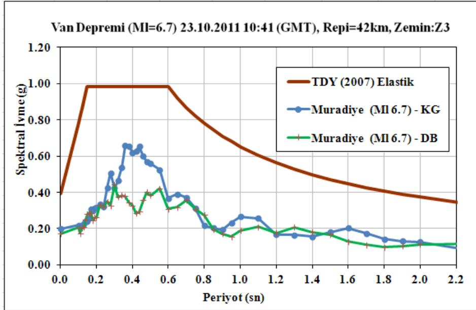
Figure 15.1: Compare with Muradiye station NS and EW component response spectrum and TDY 2007 design spectrum
