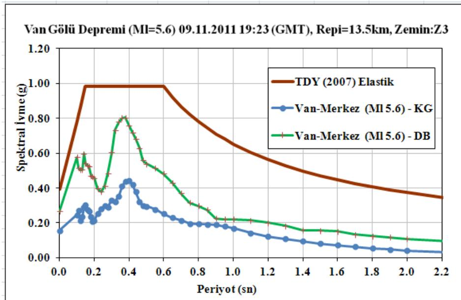
Figure 15.2: Compare with Van-merkez station NS and EW component response spectrum and TDY 2007 design spectrum.
