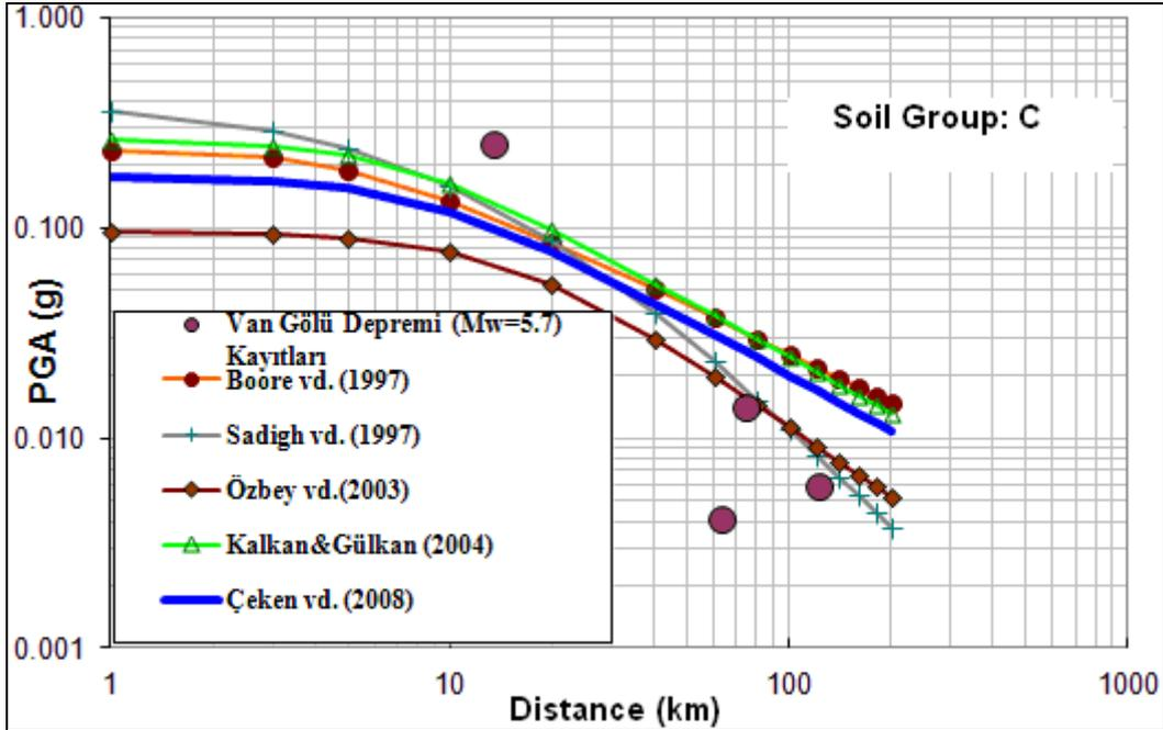
Figure 16.4: Compare with peak ground horizontal acceleration value and some attenuation relationship for 09 November 2011 Mw=5.7 Van-Edremit earthquake(soil group:C)
