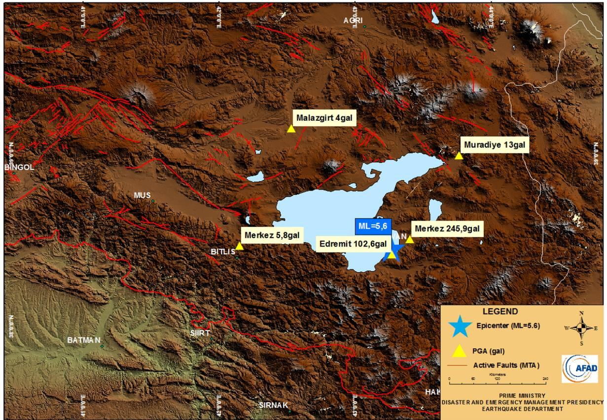
Figure 10.2: Distribution of the recorded stations and peak ground accelerations for 09 November 2011, ML=5.6 Van-Edremit Earthquake.
