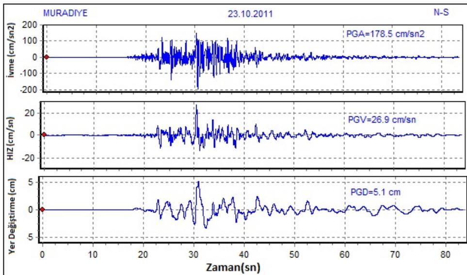
Figure 11.1: NS direction acceleration, velocity and displacement components for 23 October 2011, MI=6.7 Van-Merkez Earthquake (Muradiye station)
