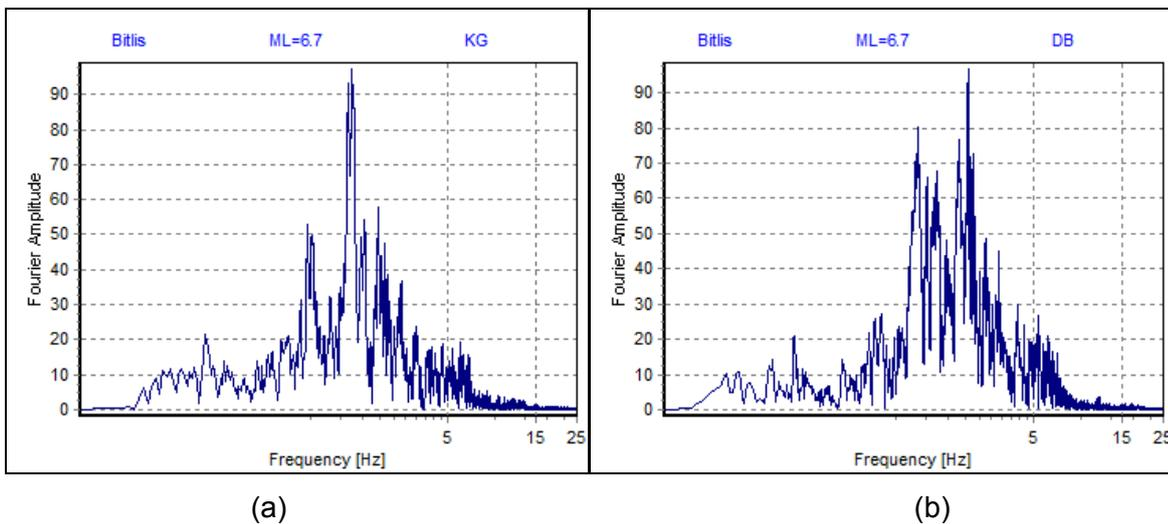
Figure 13.2: Fourier spectrums of 23 October 2011,  $M_L=6.7$  Van-Merkez earthquake
