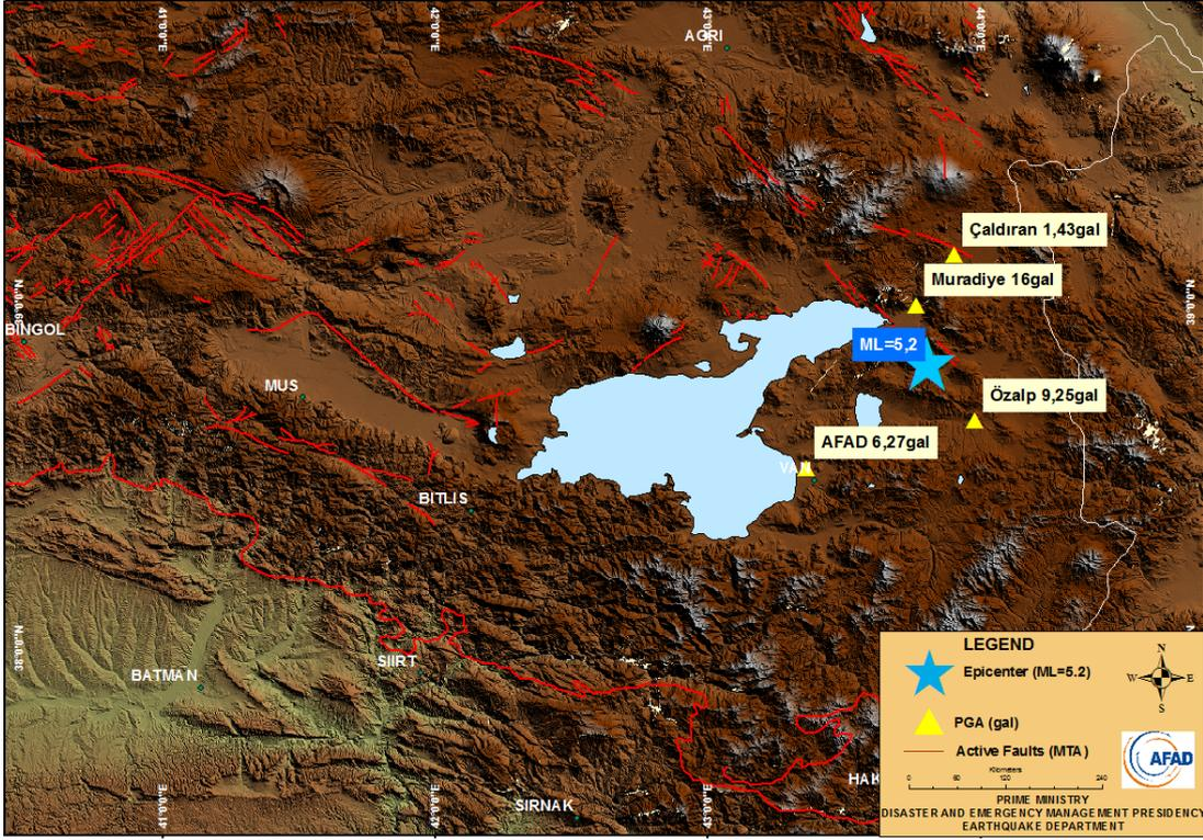
Figure 10.3: Distribution of the recorded stations and peak ground accelerations for 18 November 2011, ML=5.2 Van Muradiye Earthquake.
