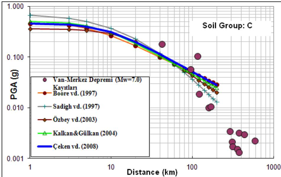
Figure 16.2: Compare with peak ground horizontal acceleration value and some attenuation relationship for 23 October 2007  $M_w=7.0$  Van-Merkez earthquake(soil group:C)
