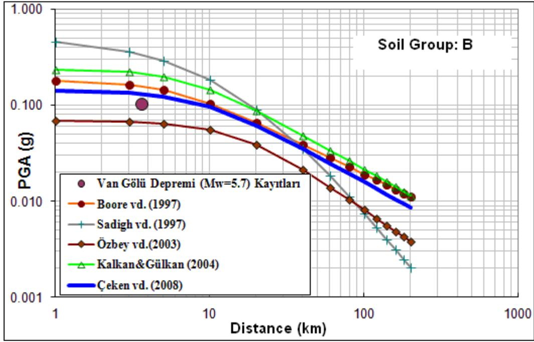
Figure 16.3: Compare with peak ground horizontal acceleration value and some attenuation relationship for 09 November 2011 Mw=5.7 Van-Edremit earthquake(soil group:B)
