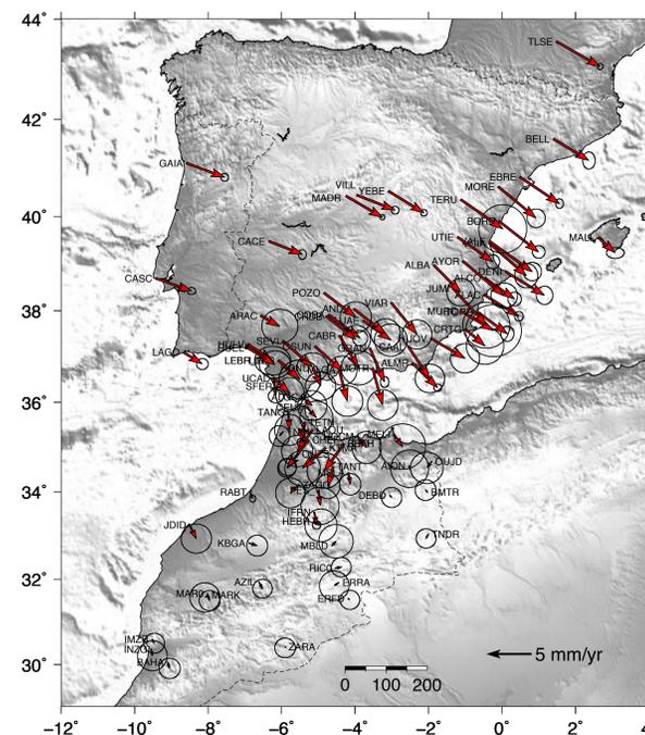
**Figure 2:** GPS site velocities with respect to Africa and 95% confidence ellipses.
