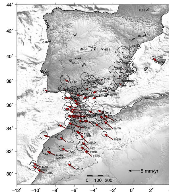
**Figure 3:** GPS site velocities with respect to Eurasia and 95% confidence ellipses.
