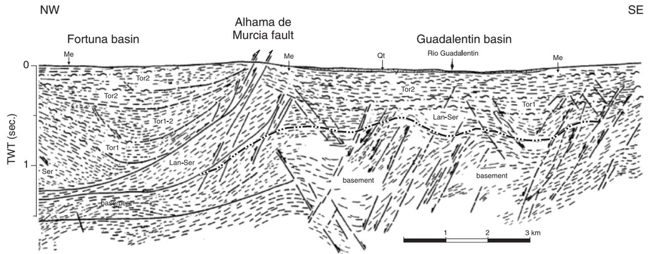
Fig. 13. Seismic profile across the Fortuna Basin, the Alhama de Murcia fault zone and Guadalentín Basin. Modified from Amores *et al.* (2001). For location see Fig. 10. Abbreviations: Lan-Ser—Langhian-Serravallian deposits; Tor1, Tor2, lower and upper Tortonian sediments; Me, Messinian sediments; Qt, Quaternary sediments.
