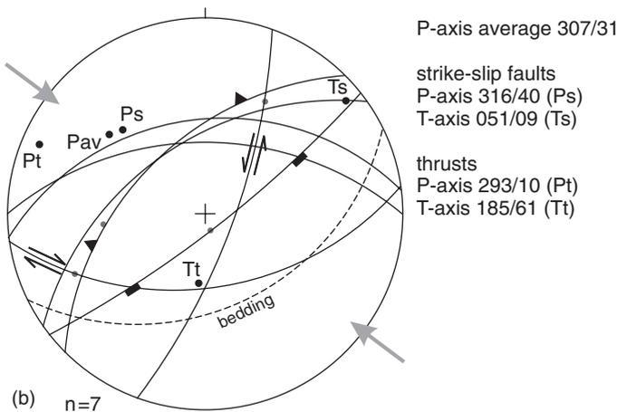
Fig. 14. (a) Exposure of the Alhama de Murcia fault northeast of Puerto Lumbreras, carrying Alpujarride rocks of the Sierra de las Estancias towards the SE onto upper Tortonian marls. For location see Fig. 10. (b) Stereographic projections (equal area, lower hemisphere) showing orientations of reverse and strike-slip faults in Miocene–Quaternary sediments and basement rocks in the Alhama de Murcia fault zone near Puerto Lumbreras. *P*- and *T*-axes as defined in Fig. 8.
