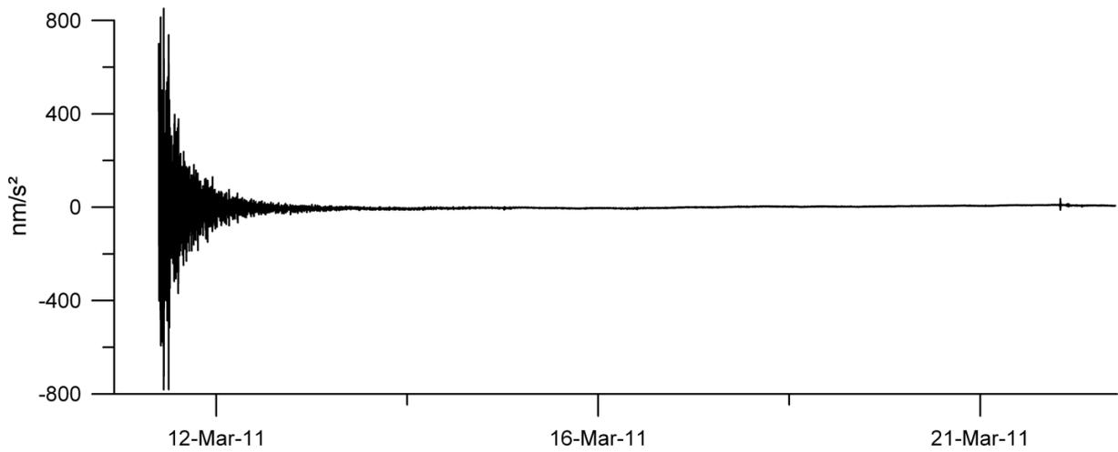
Figure 1. Time series of the superconducting gravimeter GWR-C021 of Membach, after the Mw=9.0 Tohoku earthquake. Data are low pass filtered at 200 s period.
