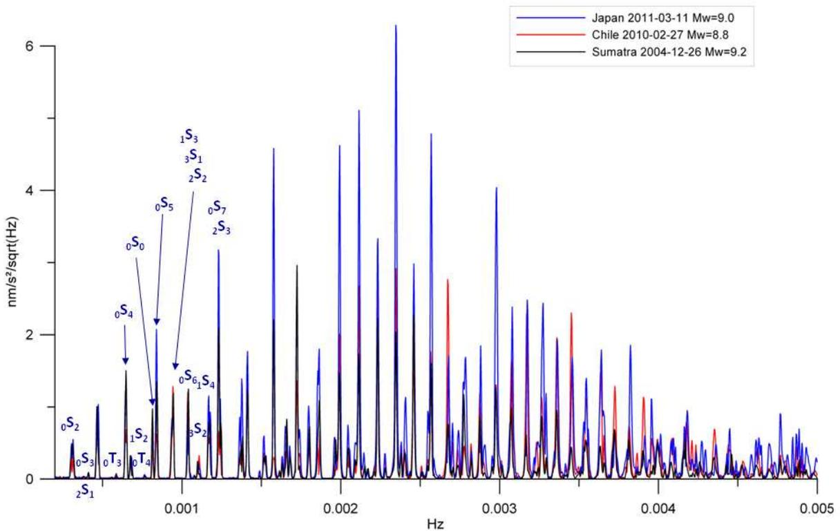
Figure 2: Spectra of the times series from the superconducting gravimeter of Membach GWR C021. This shows the excitations of the different eigenfrequencies of the Earth after 3 different earthquakes, for frequencies shorter than 5 mHz (or periods longer than 200 seconds). The “football” mode  ${}_0S_2$  is the slowest one (period  $\sim 54$  minutes).
